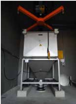
Figure 2: Replaceable container for PAC storage
